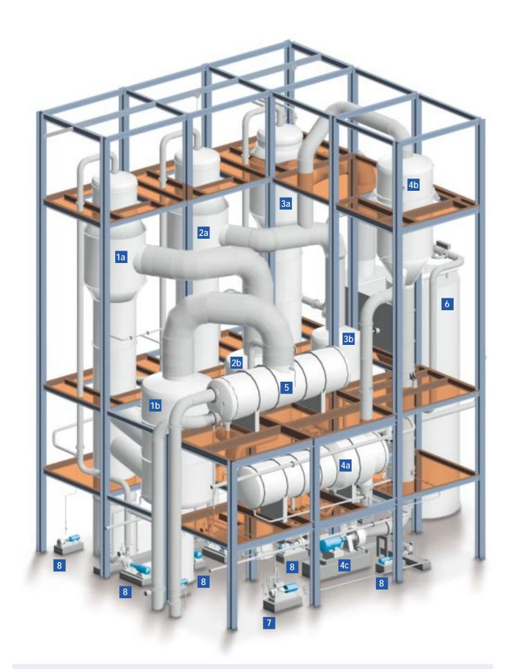
1a, bFalling film evaporator with centrifugal separator2a, bFalling film evaporator with centrifugal separator3a, bFalling film evaporator with centrifugal separator4a, b, cForced circulation evaporator with flash vessel/<br/>gravitational separator and circulation pump
