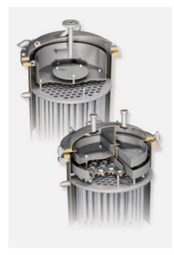
Two examples of suitable distribution systems, above: Perforated bowl, below: Tubelet
