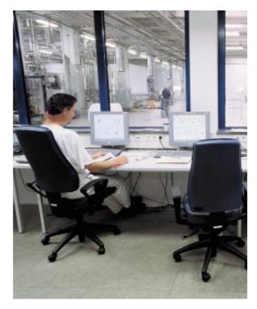
The processes can be centrally operated and monitored on the screen by means of a bus system. Set points and other key parameters are entered into the fields shown on a graphic display. The plant is self-monitored and is automatically switched to a safe mode in the event of operating trouble. The use of a multiple operator station system increases the availability.
